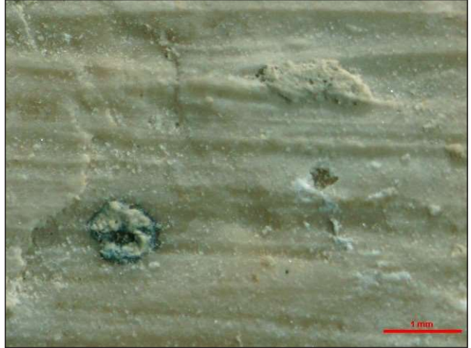
Figure 15.11. Optical microscopy evaluation of binder reverse, x15 magnification.
